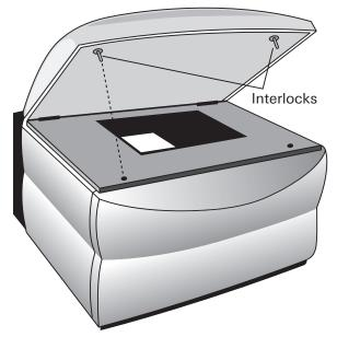
Figure 1-4. Location of interlocks on the Odyssey<sup>®</sup> CLx instrument bezel.
