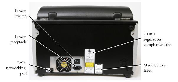
Figure 2-3. Closeup of the Odyssey<sup>®</sup> CLx Imager rear panel showing the power receptacle and LAN port (use only the supplied networking cable). Also shown are the CDRH regulation compliance label, the manufacturer label and the power switch. The power switch can be left in the 'on' position. Note: The appearance of your instrument's back panel may vary slightly from the one shown.
