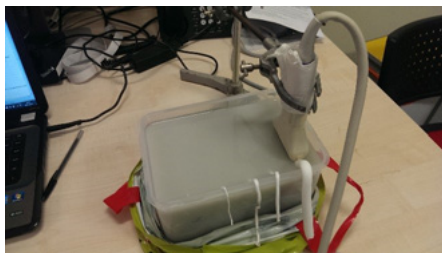
Figure showing ultrasound test object with pipes of varying dimensions and elastic modulus being scanned.
