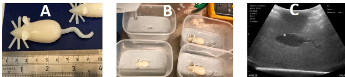
Figure A showing manufactured agar mice, B. mice being embedded within tissue mimicking material and C. ultrasound scan of one of the agar mice within the test-object.
